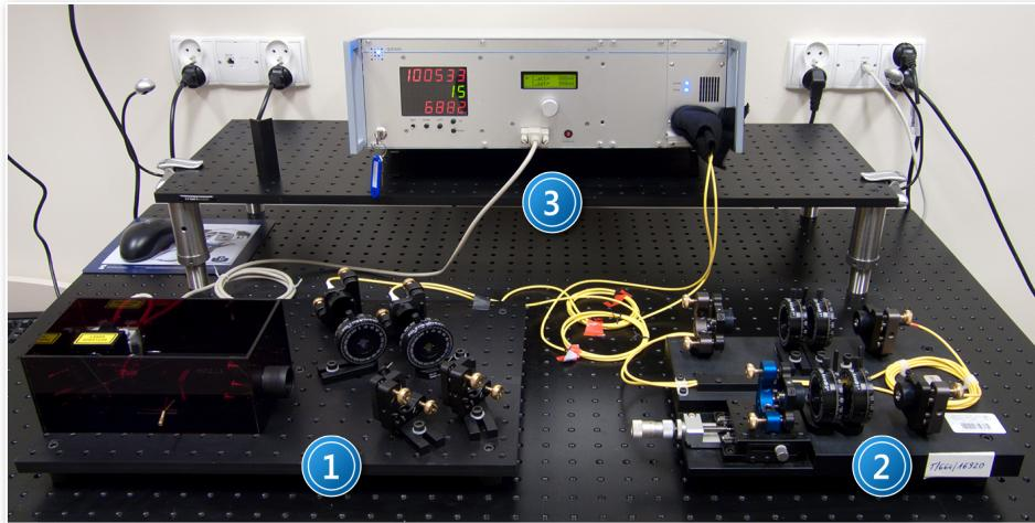
*Picture 1. Experimental setup to study the properties of polarisation-entangled photon pairs: 1 – system for demonstrating entanglement visibility; 2 – system for studying two-photon interference; 3 – multi-function unit: power supply – controller – single-photon detector.*
