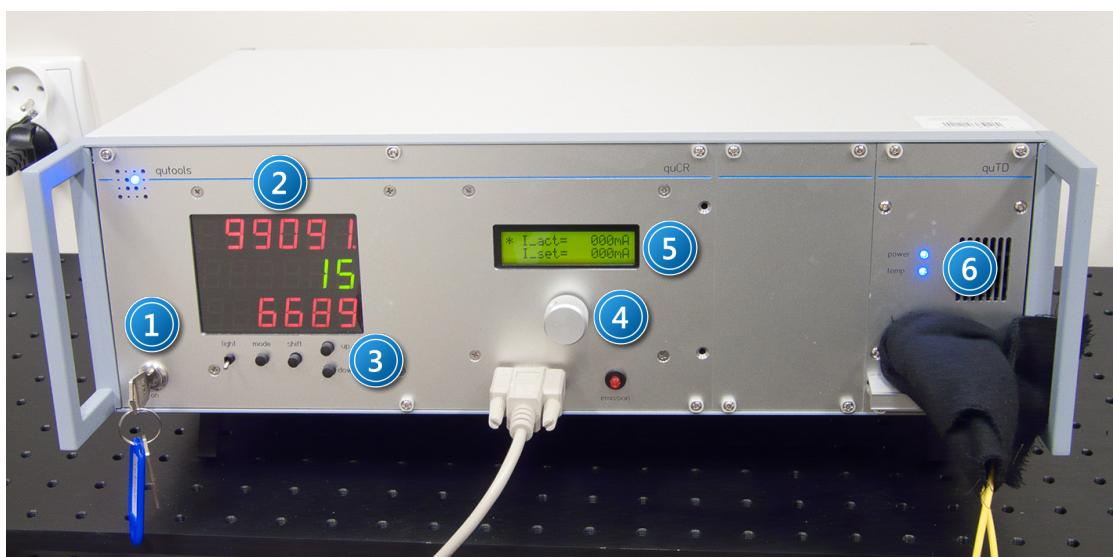
*Picture 5. Measuring unit – controller, multifunction power supply, single-photon detector: 1 – main switch; 2 – count display; 3 – count function keys; 4 – laser settings dial; 5 – laser settings display; 6 – APD module indicators.*
