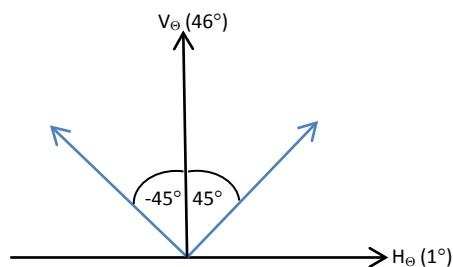
*Figure 4. The direction of the pumping beam to ensure an equal number of photons with polarization H and V (with angle  $23,5^\circ$  for the half-wave plate 3 in Picture 2).*
