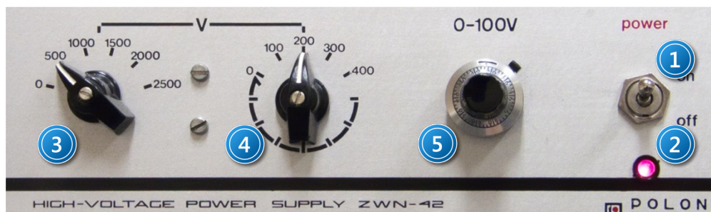
Picture 4. High-voltage power supply control panel "POLON ZWN-42", to power the Kerr cell: 1 – power switch (before turning on power, make sure that the knobs are set to "0"!), 2 – control LED, 3 – coarse adjustment knob with increments of 500 V, 4 – coarse adjustment knob in increments of 100 V, 5 – fine adjustment knob ranging from 0 to 100 V
