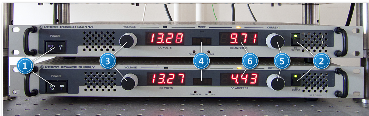
Picture 3. Electromagnet power supply control panel: 1 – “POWER” switch; 2 – “DC OUTPUT” mode switch; 3 – “VOLTAGE” control knob; 4 – maximum voltage control window; 5 – “CURRENT” control knob; 6 – displays the current of the generated electricity.
