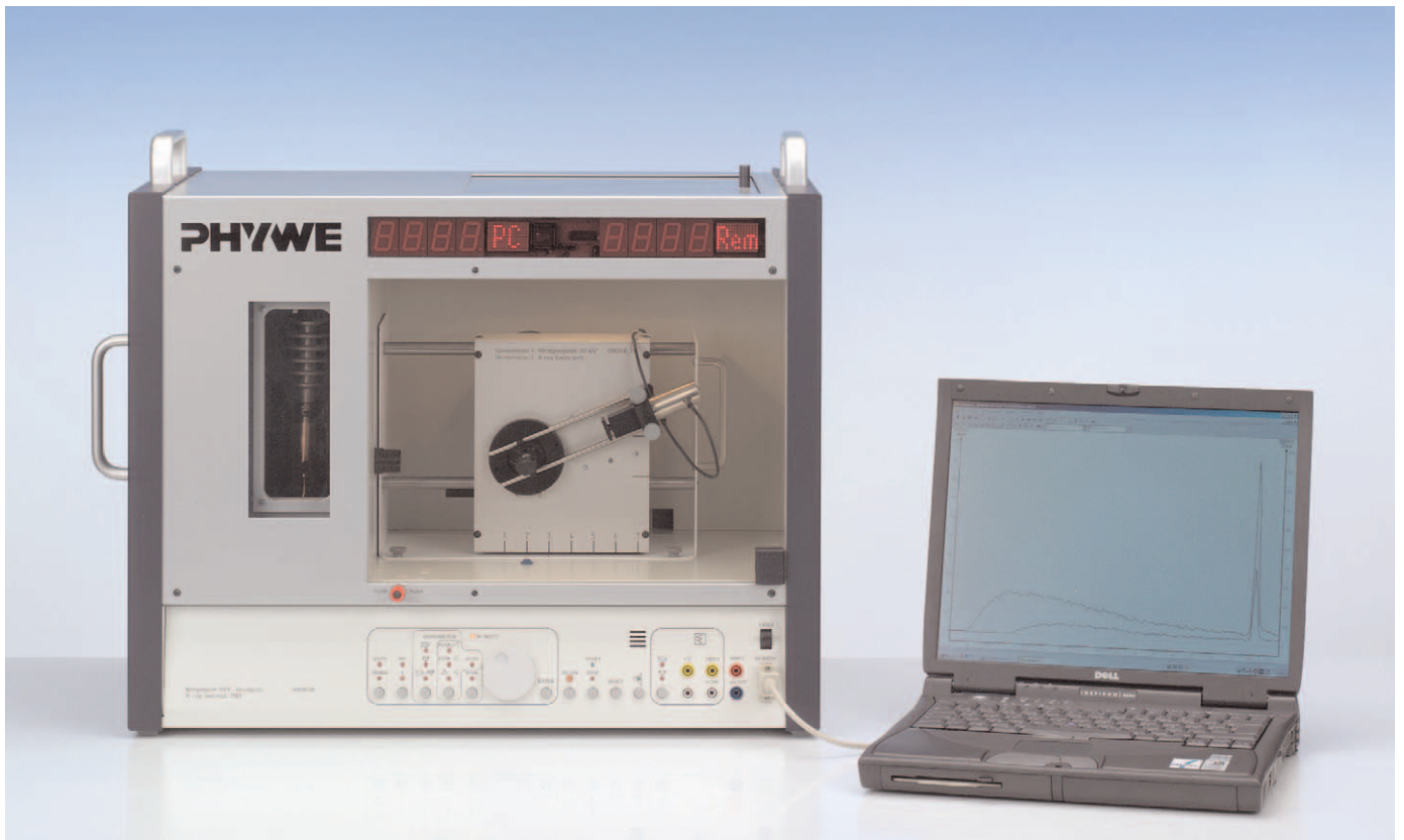
Fig. 1: Experimental set-up for the analysis of X-ray energies
