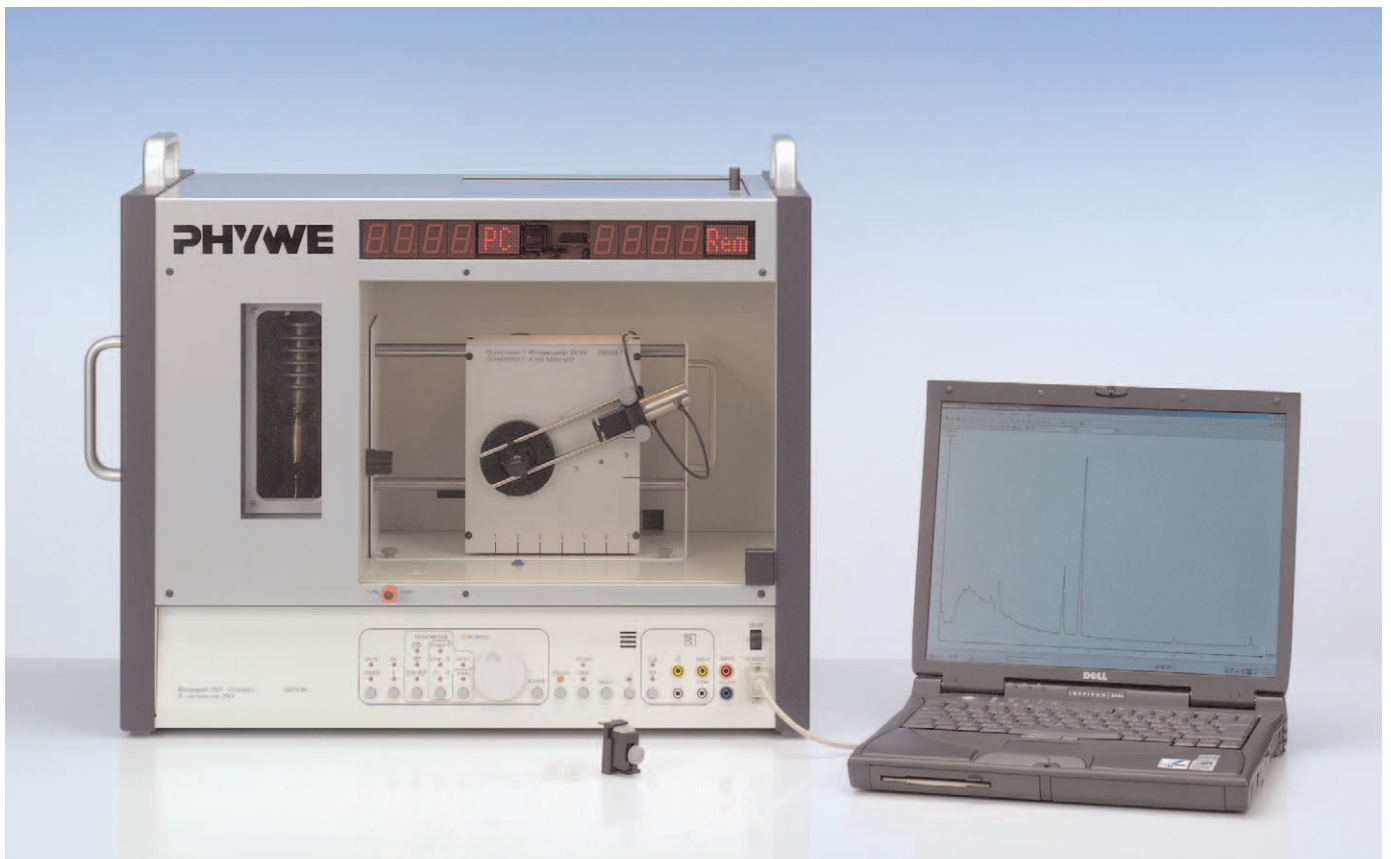
Fig. 1: Experimental set-up for the examination of the structure of NaCl monocrystals
