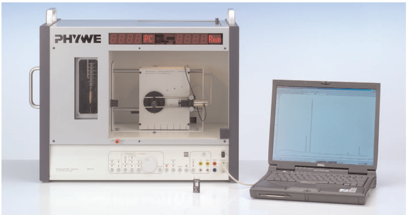
Fig. 1: Experimental set-up for the analysis of X-rays
