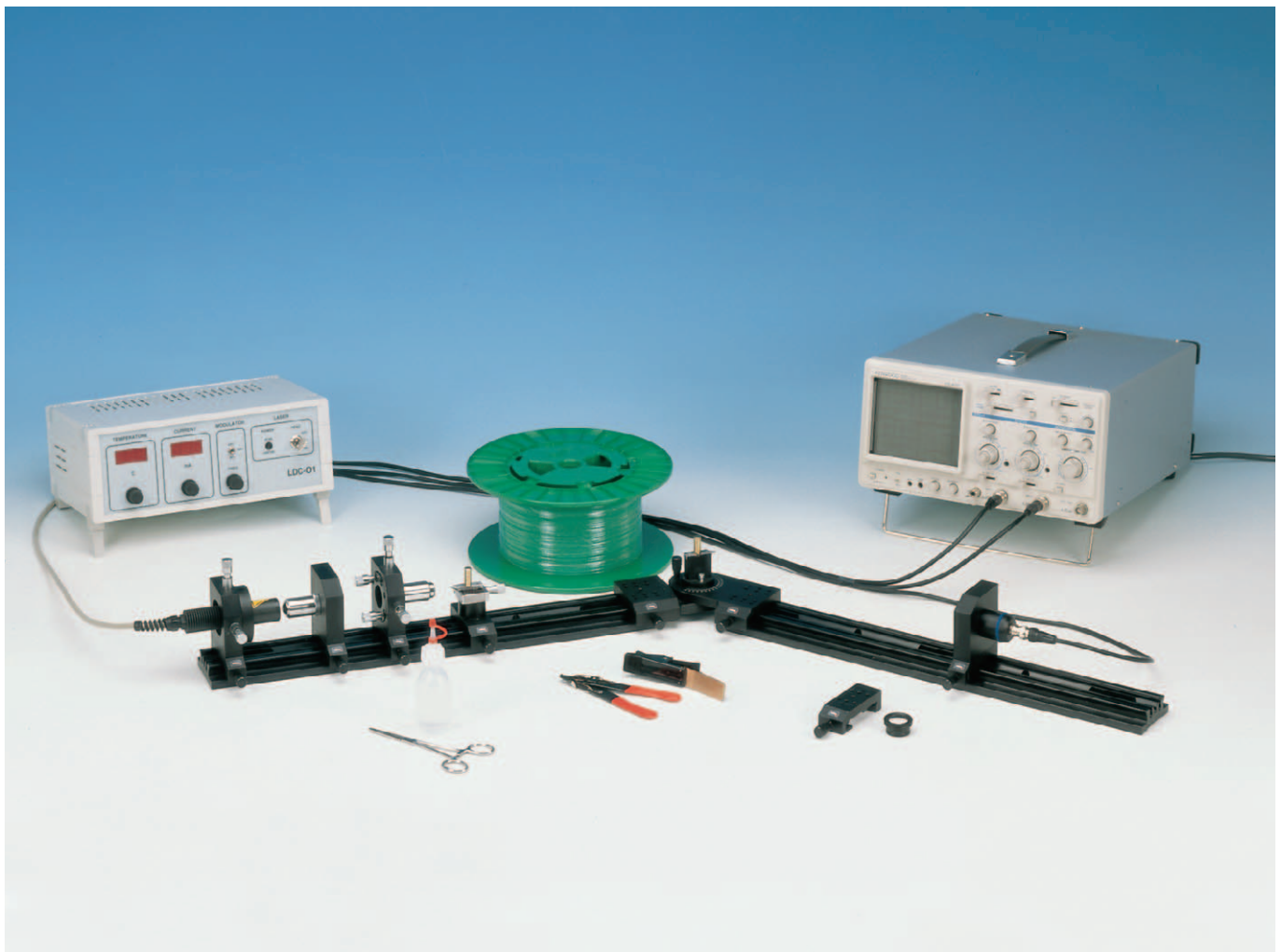
Fig. 1: Experimental set-up: Fibre optics with monomode fibre.
