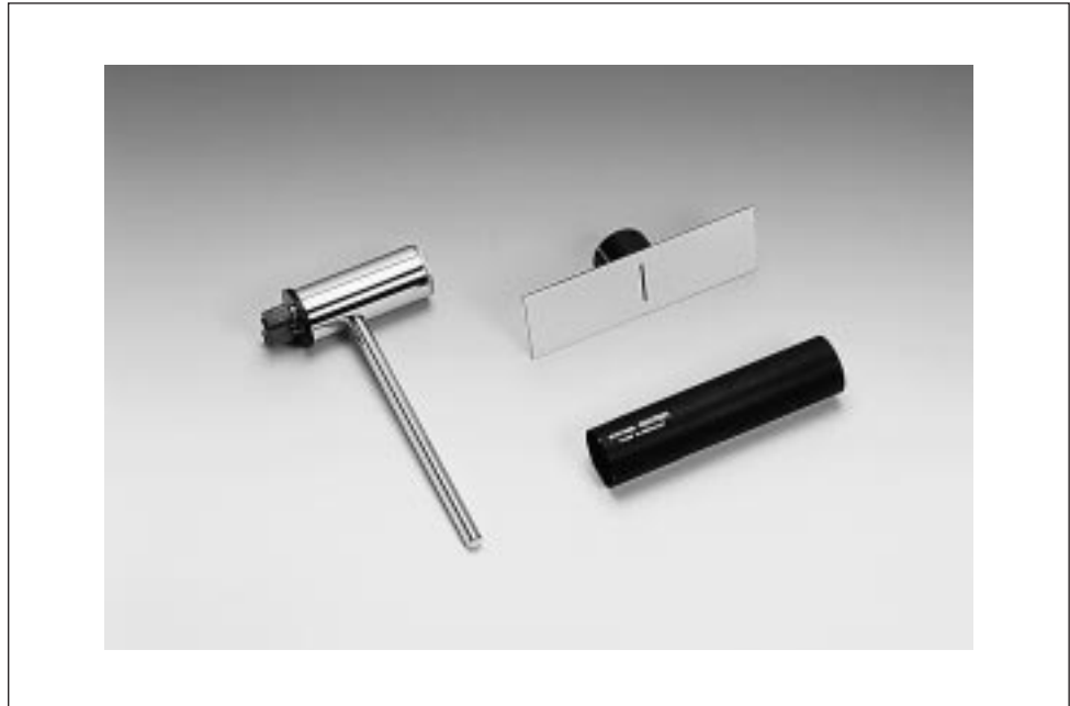
Fig. 1: Moll type thermopile with shielding tube 08479.01 and slit 08479.02
