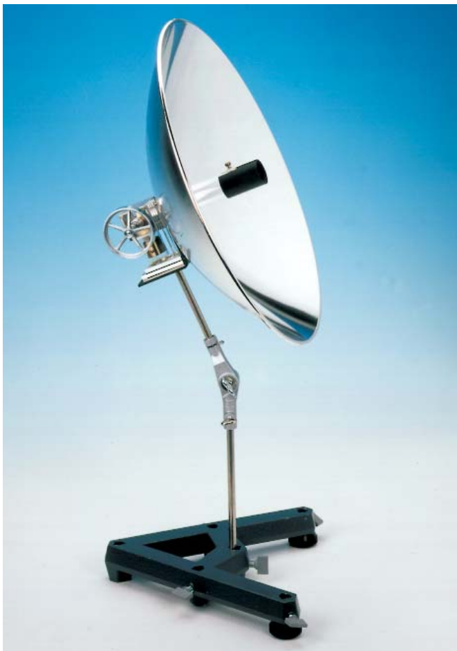
Fig. 12: Stirling engine with accessories for heating by the sun.
