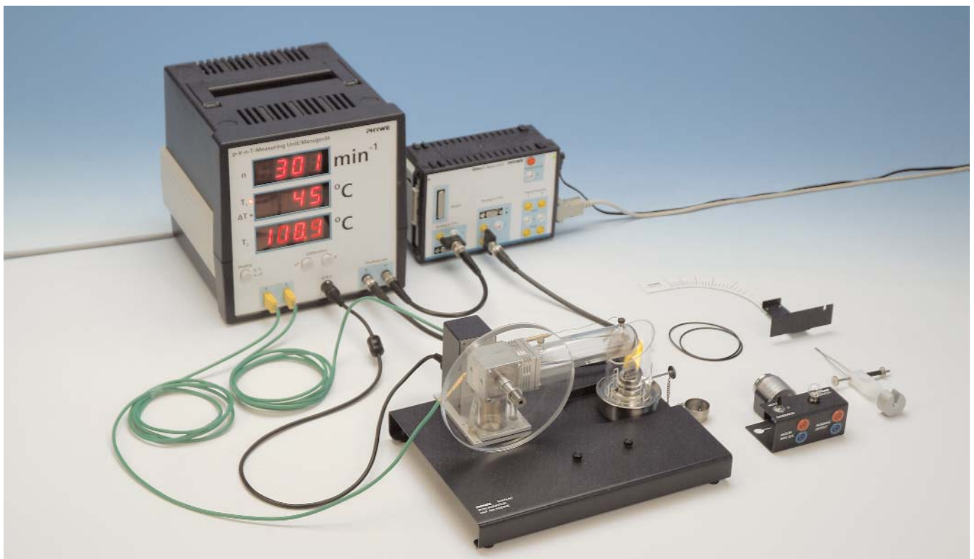
Fig. 1: Experimental set-up: Stirling engine.
