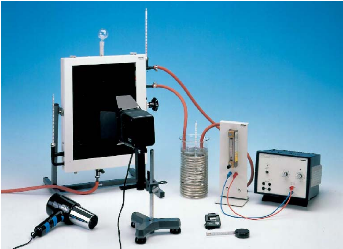
Fig. 1: Experimental set-up: Solar ray Collector.
