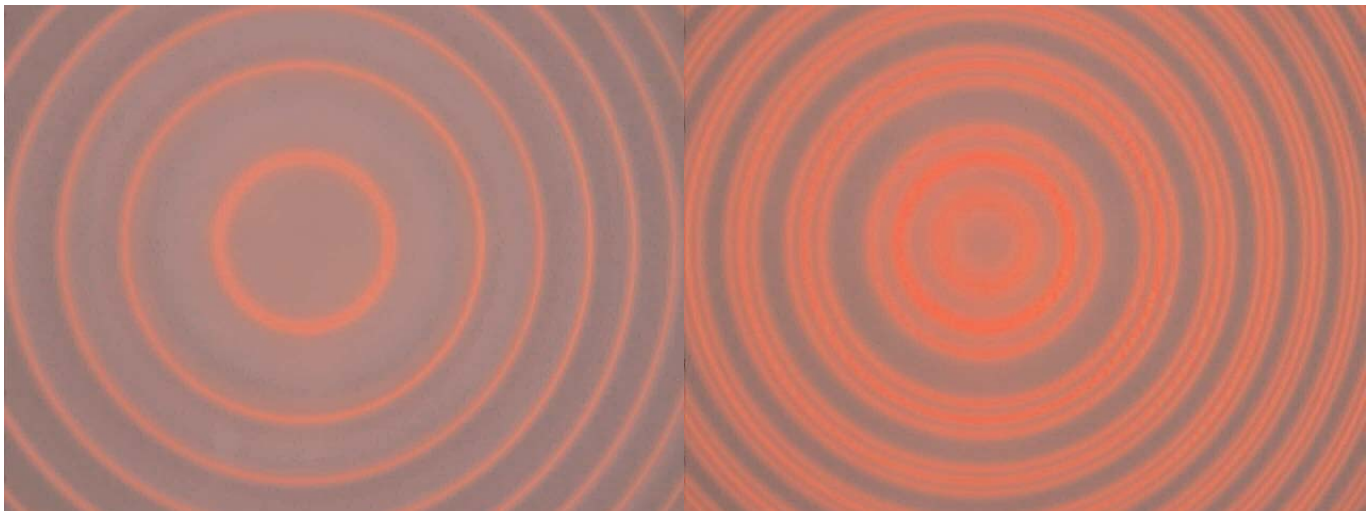
Fig.10: Normal Zeeman effect: Interference pattern without polarization filter for no coil current and for 5 A coil current. On the left there is one ring per order of interference, on the right there are three rings per order of interference
