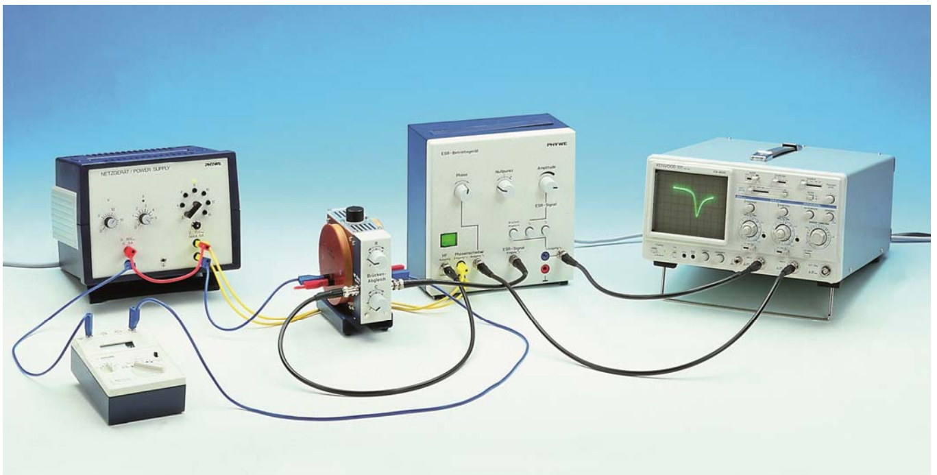
Fig. 1: Experimental set-up for determining characteristic curves.
